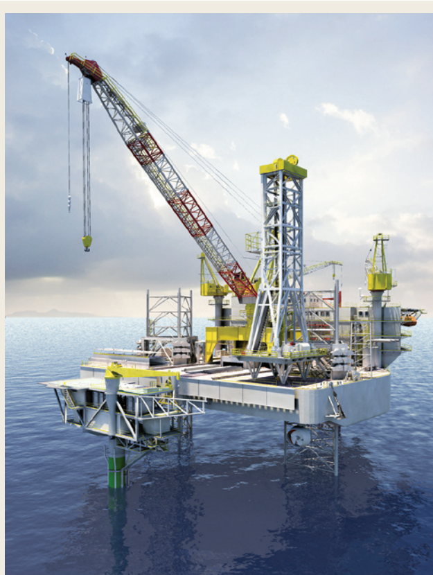
Fig. 1. The self-propelled ESV hybrid jackup can position itself with DP-1 capability. The onboard moveable pedestal crane can hoist 110–300-ton (100–272 metric ton) loads within a 160-ft (48-m) radius. A workover derrick may be deployed on cantilever or on well-platform beams.
